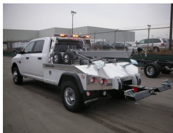
2012 CHEV 3500 DIESEL CREW CAB C/W JERR- DAN HPL 35 WRECKER WHEEL LIFT & 4 TON BOOM IN PRODUCTION
