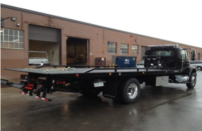
2013 INTERNATIONAL 4400 10 SPEED C/W 24' 7.5 TON STEEL JERR-DAN CARRIER, WHEEL LIFT & SIDE RECOVERY SYSTEM
